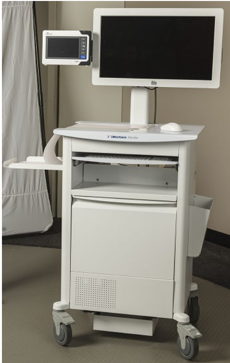
Figure 2 Example of a Stress Cart with the Z200+ Thermal Writer, Tango M2, and Touch Monitor
